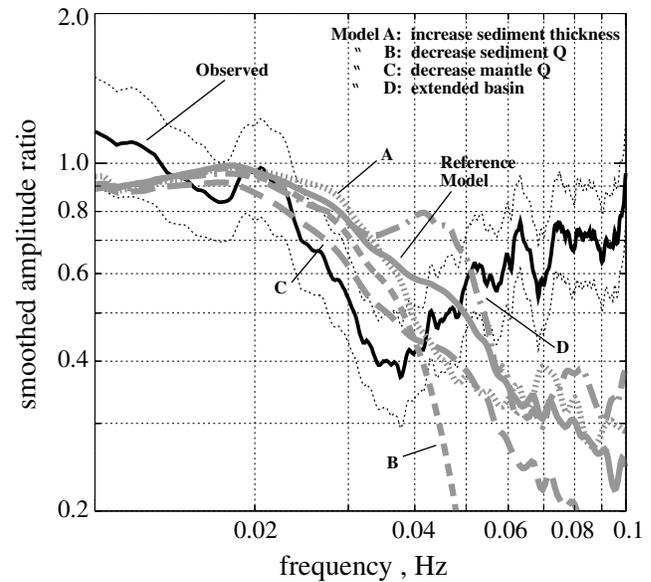
Figure 3. Amplitude ratios for Rayleigh waves propagating across the South Caspian Sea. Black line and thin dotted lines are the average ratio and one-standard-deviation error bars based on 14 sets of observations for stations KAT and LNK. Thick gray lines are amplitude ratios from FD modeling: (1) solid-reference model, (2) dotted-model A, (3) short dash-model B, (4) long dash-model C, and (5) dash-dot-model D.
