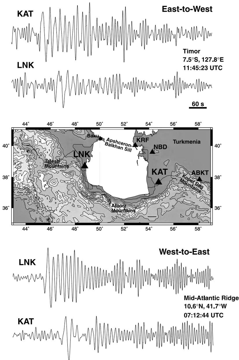
Figure 1. The middle part of the figure shows a map with locations of the broadband digital stations in the region surrounding the South Caspian basin. Seismograms for two earthquakes lying on the same great circle path as the stations are shown above and below the map. The lower pair of seismograms are from an earthquake on the Mid-Atlantic Ridge; the upper pair of seismograms are from an earthquake in Timor. All seismograms are plotted at the same amplitude scale.
