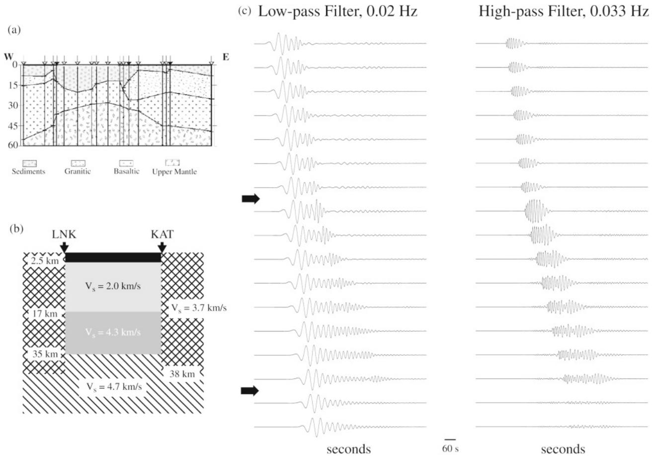
Figure 2. (a) The South Caspian basin model of Mangino and Priestley (1998). (b) The simplified South Caspian basin shear-wave model used in the FD calculations. (c) Synthetic surface-wave record sections for two passbands: up to 0.02 Hz at left, and 0.033 Hz and above at right. The large arrows denote the location of the basin boundaries. All seismograms in a record section are plotted at the same amplitude scale, but the two record sections have different scales.
