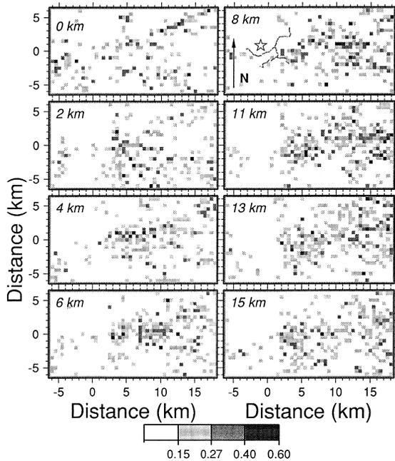
Fig. 8. Emission images of the medium at different depths for the transverse component of seismic noise before the onset of P-wave for earthquake 4. Depth is marked on each image. The density scale shows the same as mentioned in the caption of Fig. 5. Star shows the epicenter of earthquake 4.
