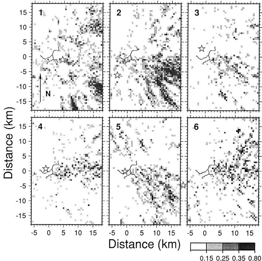
Fig. 6. Emission images of the medium at 11 km depth for the transverse component of seismic noise before the onset of P-wave for earthquakes 1–6 in Table 1. The density scale shows the same as mentioned in the caption of Fig. 5. Stars show the epicenters of earthquakes.
