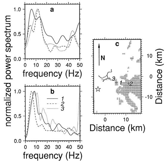
Fig. 9. Normalized power spectra of transverse component of seismic emission for noise samples before the onset of P-wave of earthquake 2: (a) for near-surface sources ( $H = 0$  km), (b) for deep-seated sources ( $H = 10$ – $13$  km) within regions studied, (c) shows the location of active volume at 10–13 km depth, numbers 1–3 mark position of focused points and corresponds to numbers of curves on (b), respectively. Star shows the epicenter of earthquake 2.
