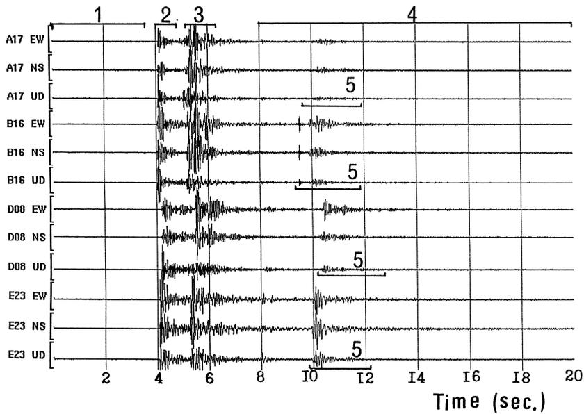
Fig. 2. Sample velocity seismograms of local earthquake 3 from Table 1 for stations A17, B16, D08 and E23. Time window used for reconstruction of emission images: (1) for seismic noise, (2) for direct P-waves, (3) for direct S-waves, (4) for coda, and (5) for reflection phase from a magma body.
