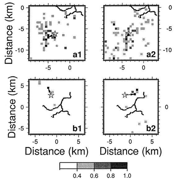
Fig. 4. Images of sources for direct waves: (a1) and (a2) earthquake 2 for P- and S-waves, respectively and (b1) and (b2) for earthquake 3 for P- and S-waves, respectively. Time window is 0.85 s for P-waves and 1.00 s for S-waves. The density scale shows the same as mentioned in the caption of Fig. 3.
