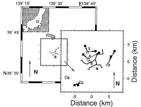
Fig. 1. Nikko-Ashio area, Honshu, Japan. Configuration of the seismic array and the images of the hypocenters of earthquakes 1–6 in Table 1 (a) Array geometry, open stars are earthquake epicenters according to the catalog; the black squares are source images from P-waves; black circles are source images from S-waves.
